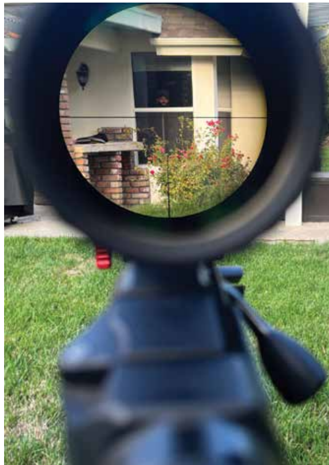
This photo is taken from 25 yards @ 6x magnification through the same FFP scope. The field of view is much smaller than at 3x.
